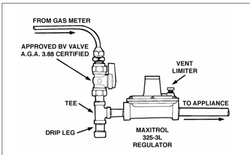
At supply pressures above 2-psi, the new standard requires the use of an over-pressure protection device (OPD) for use with the regulator. (See below.)
