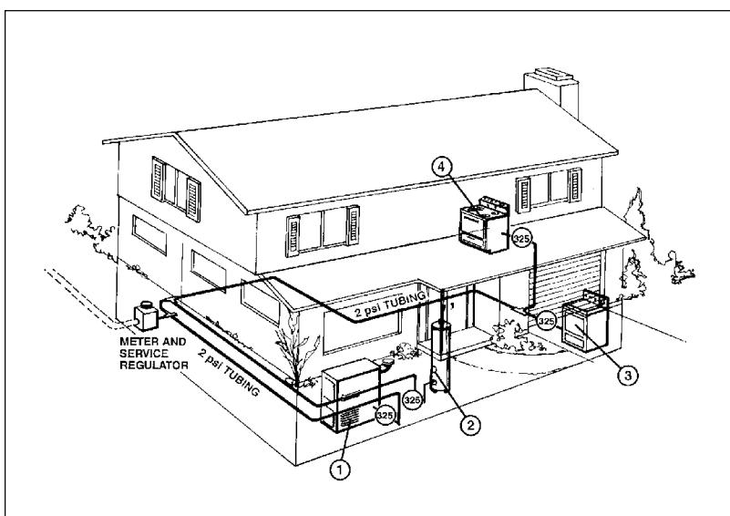
Typical 2-psi house piping system using Maxitrol 325 Series gas pressure regulators — Use one with each appliance:
